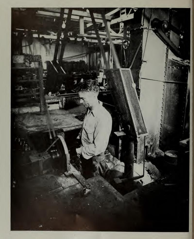
However, before the cap is fastened to the bearing end of the rod any ragged edges of babbitt which may have adhered where the shims separated the cap from the bearing end of the rod are removed by holding the open face of the cap or the open face of the bearing end of the rod against the revolving sandpaper disc as shown above.
